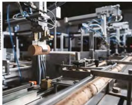
NDTech artificial cork sniffer in action.
