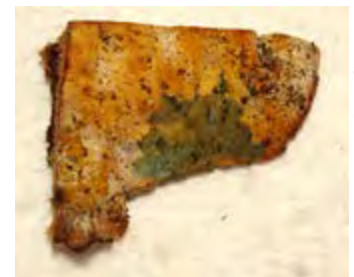
Specimen tested positive with tincture of Guaiac resin, turning green, showing it's a white rot fungus.
