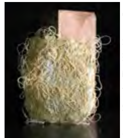
Mycelium spores growing on linen yarn for potential construction materials.
