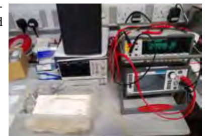
Unlike the mock-up, the real mushroom computer resides in a plastic container.
